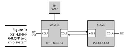
Links marked NC are not required by the system topology. The I/O pins that overlap these xCONNECT links can be used for other purposes.
