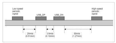
Figure 7-1 USB trace separation showing low speed signal, a differential pair and high-speed clock
