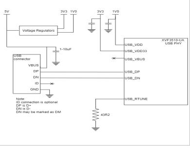
Figure 3-1 Bus-powered USB design
