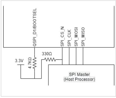
Figure 3-3 XVF3510 SPI slave boot configuration
