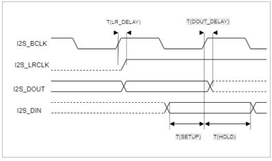
Figure 6-2 I2S master timing
