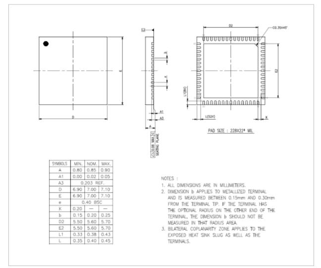
Figure 8-1 QFN60 package dimensions
