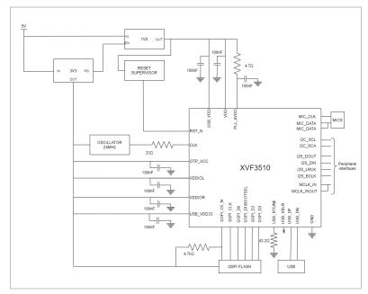
Figure 1-3 Essential components of a XVF3510-UA application booted from a QSPI flash
