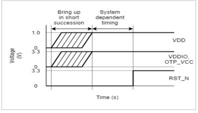
Figure 4-1 Sequencing of power supplies and RST\_N
