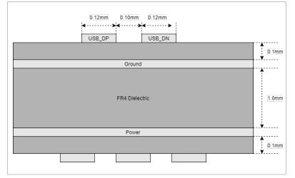
Figure 7-2 Example USB board stack
