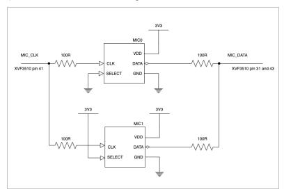
An example microphone circuit is shown in the figure below:
