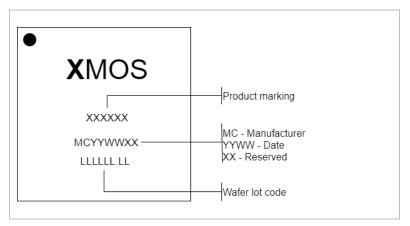
Figure 8-2 Part marking scheme
