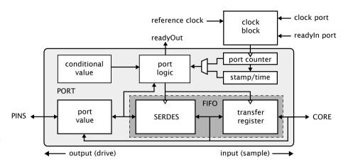
Figure 4: Port block diagram
