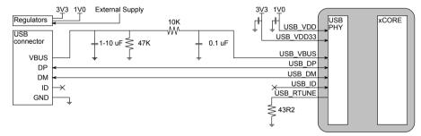
Figure 12: Self powered USB-device
