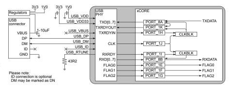
Figure 11: Bus powered USB-device
