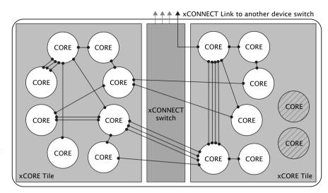
Figure 6: Switch, links and channel ends
