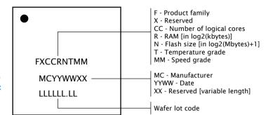
Figure 30: Part marking scheme
