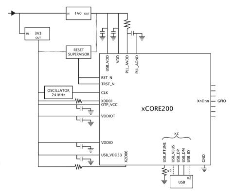
Figure 2: Simplified Reference Schematic
