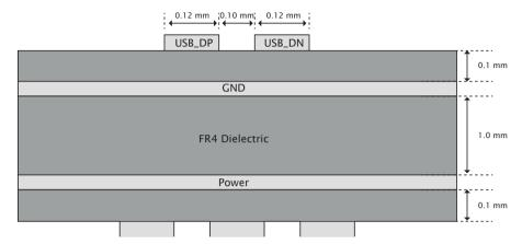
Figure 18: Example USB board stack
