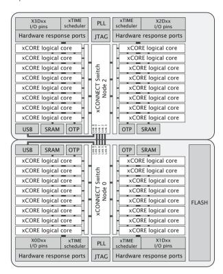
Figure 1: XUF232-512-FB374 block diagram
