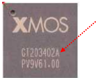
Identification of package with new 65nm embedded flash device
