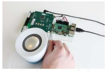
Next, load the Pi software: www.xmos.com/vocalfusion-avs Then, connect power to the Pi 'PWR IN', as above
