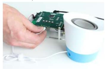
Place the speaker adjacent to and behind the mic array Note: only the left channel is active, right is muted
