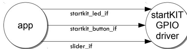
Figure 2: GPIO task diagram
