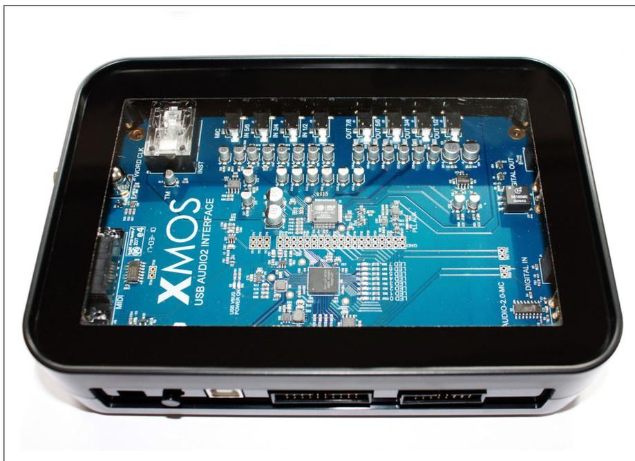
The XS1-L2 event-driven processor communicates with the USB host via a ULPI USB transceiver at the 480Mb/s high-speed rate. The XS1-L2 controls the streaming of audio data over the USB connection and direct I2S interface to the audio CODEC, digital streams and MIDI communications. Multiple additional functions (for example Mixers/DSP) can be implemented by modifications to the standard software.
