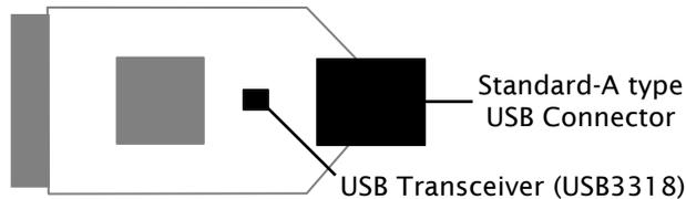
The USB connector is connected to an SMSC USB3318 high-speed transceiver using a ULPI interface. The I/O pins for the USB transceiver are mapped to ports on the processor as described in the tables below.
