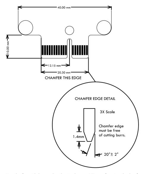
Note that for quick, low cost boards using low cost PCB manufacturing, the chamfer is not required and can be generated by hand using a file or similar.
