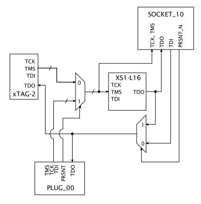
Presence detect signals are present on both the Chain connector and Square slot connectors to allow detection of a connected board and subsequent automatic switching of the JTAG chain. In a system of multiple core boards, the Master is the source of the JTAG chain so the system can only be debugged from the master. Other boards will see no devices in the JTAG chain.
