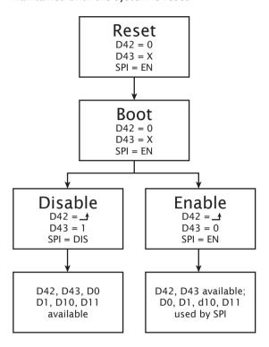
Once this sequence is completed and the selection has been latched, X0D42 and X0D43 return to performing their normal functions in the Triangle slot.
