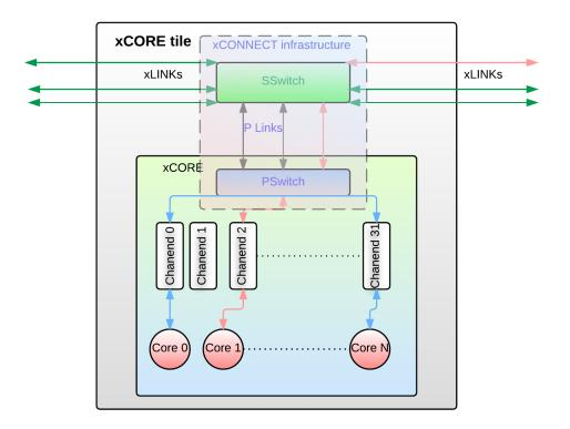
Figure 1: Block diagram of an xCORE tile
