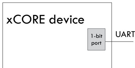
Figure 3: UART half duplex connection
