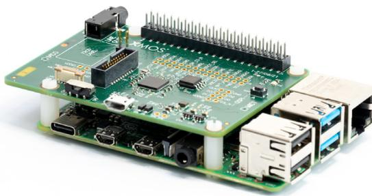
Shown assembled with Raspberry Pi (not supported) for full AVS client demonstration.
