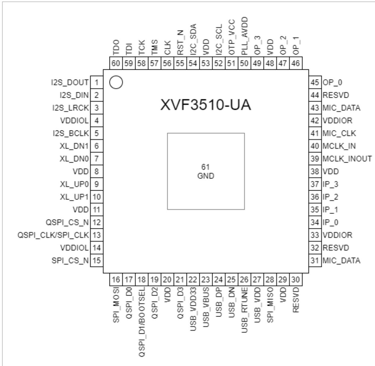
Figure 2-1 VocalFusion XVF3510-UA pin configuration
