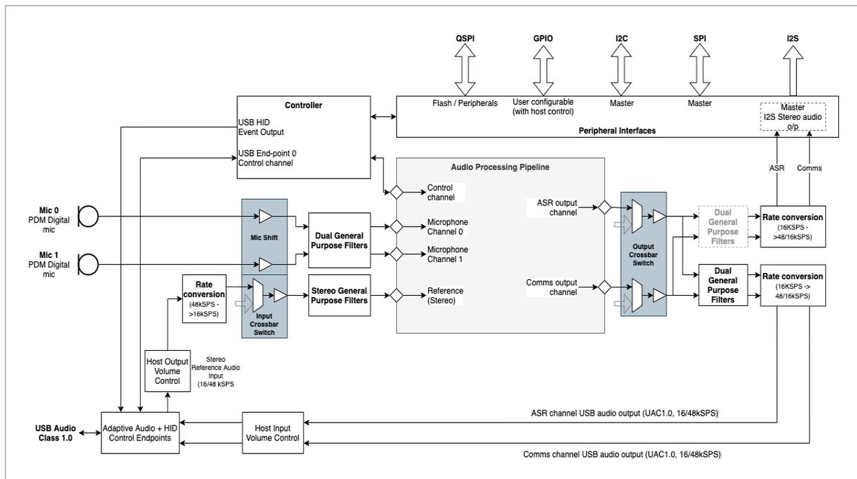
Figure 1-1 Functional block diagram of XVF3510-UA
