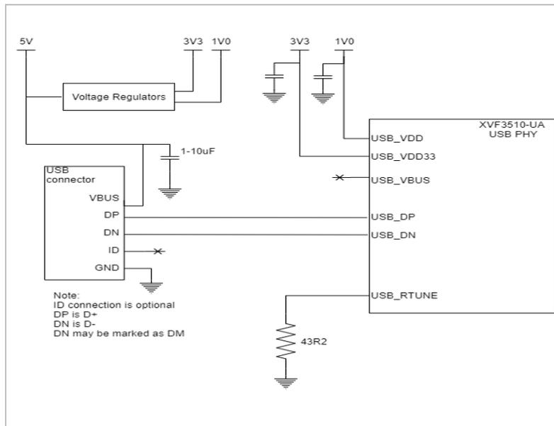
Figure 3-1 Bus-powered USB design
