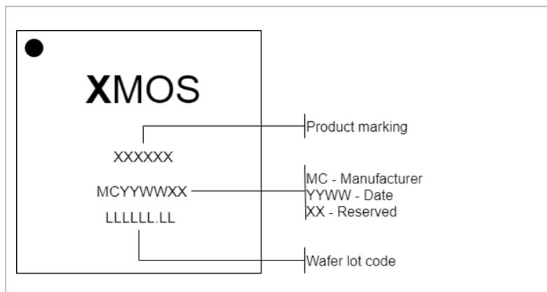
Figure 8-2 Part marking scheme
