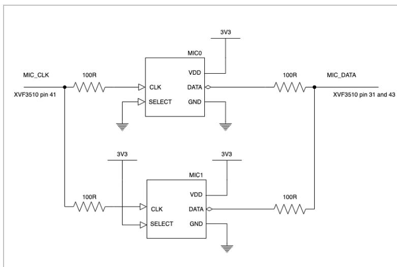
Figure 3-2 PDM microphone schematic
