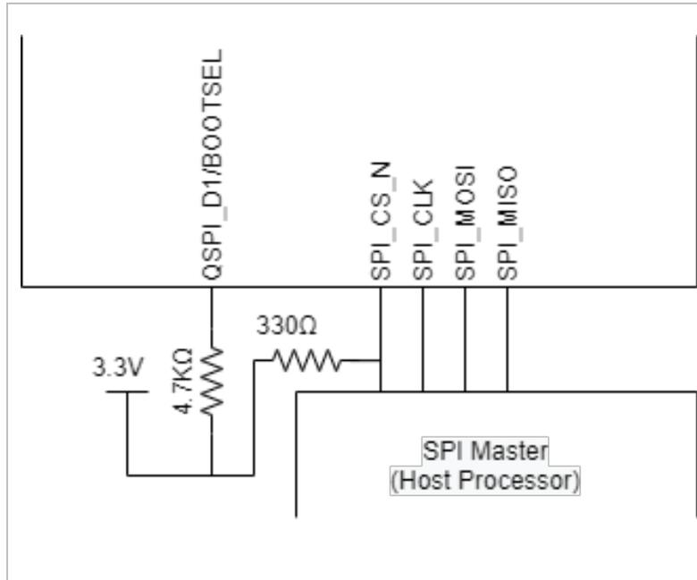
Figure 3-3 XVF3510 SPI slave boot configuration
