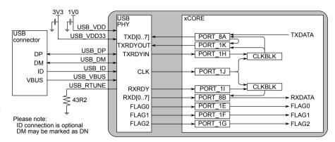
Figure 11: USB port functions
