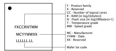
Figure 27: Part marking scheme
