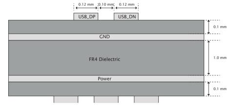
Figure 16: Example USB board stack
