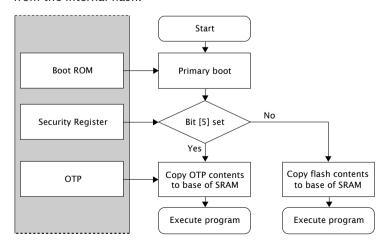
Figure 9: Boot procedure The boot image has the following format:
