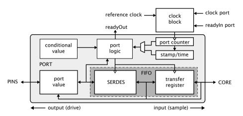
Figure 4: Port block diagram
