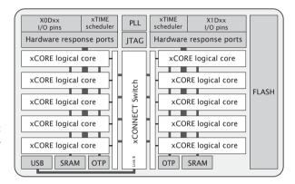
Figure 1: XUF210-256-TQ128 block diagram
