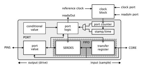
Figure 4: Port block diagram
