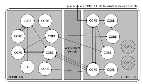
Figure 6: Switch, links and channel ends
