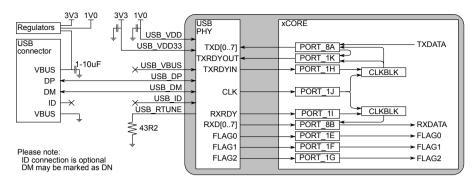
Figure 14: Bus powered USB-device
