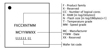
**Figure 32:** Part marking scheme
