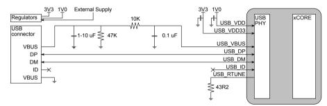
Figure 15: Self powered USB-device
