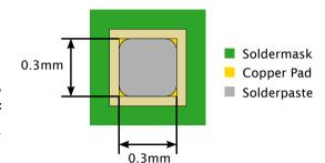
Figure 14: Solder stencil for outer pads
