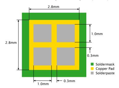
Figure 15: Solder stencil for centre pad
