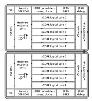
Figure 2: Block Diagram
