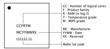
**Figure 25:** Part marking scheme
