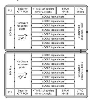
Figure 1: XS1-L Series: 4-16 core devices
