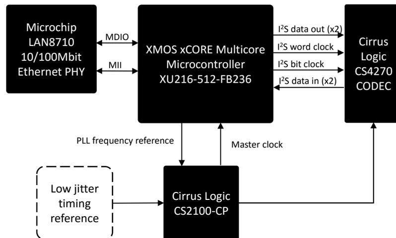
Figure 1: Block diagram of the xCORE-200 General Purpose SliceKIT hardware relevant to AVB
