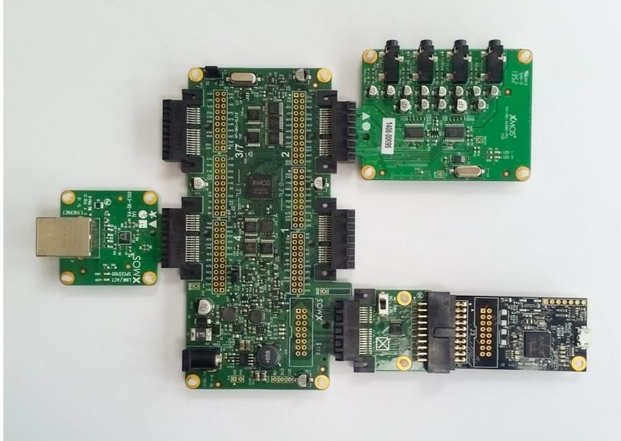
Figure 3: xCORE-200 General Purpose SliceKIT
