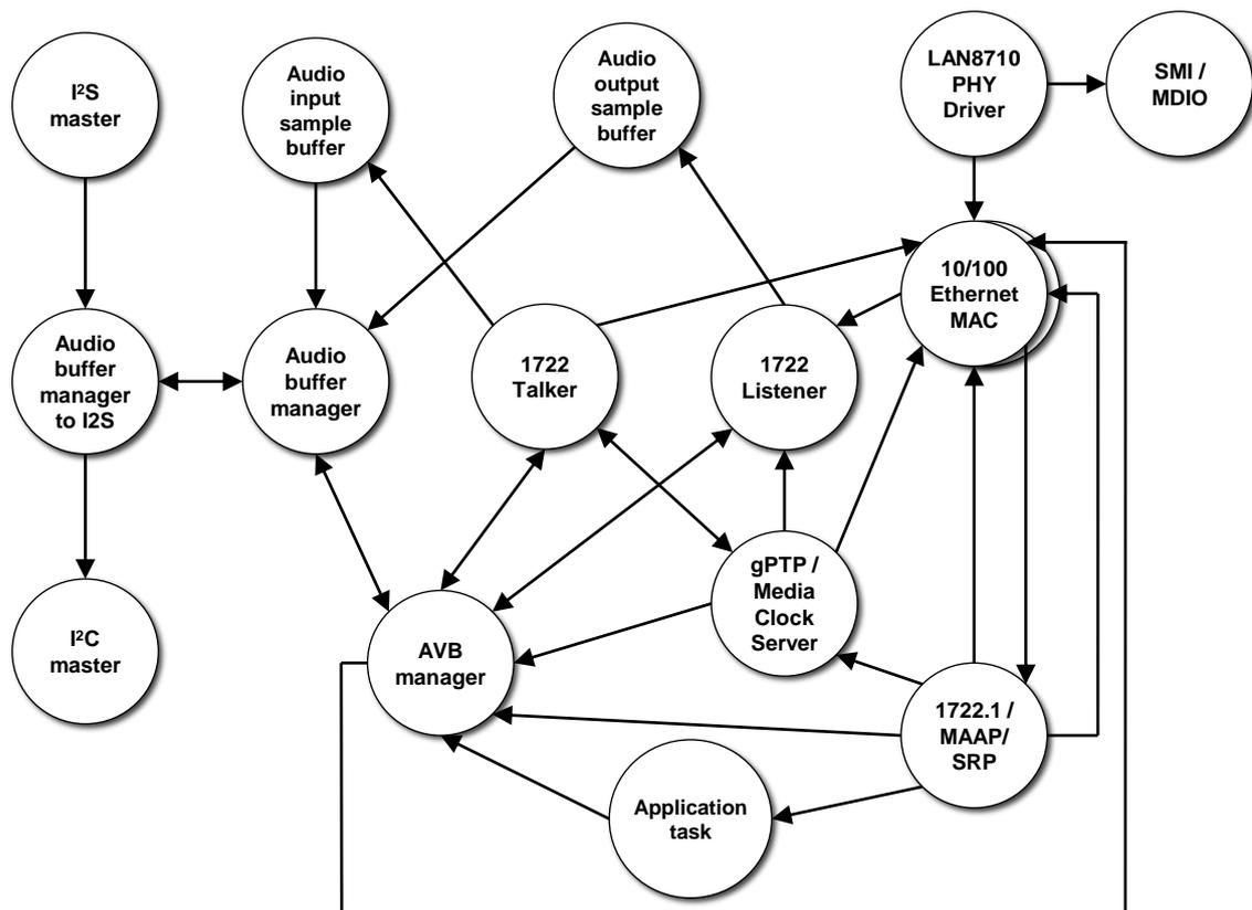
Figure 2: Task diagram of the AVB endpoint example
