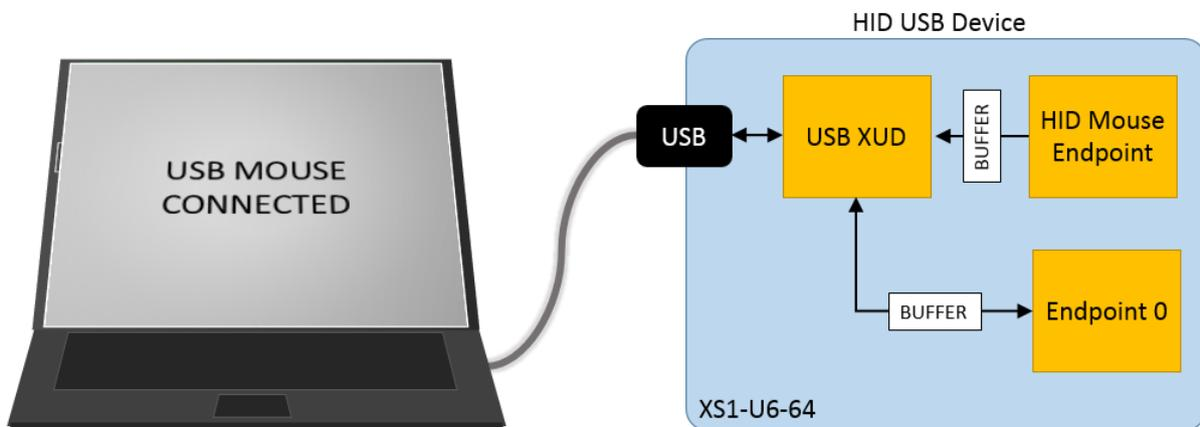
Figure 1: Block diagram of extended USB HID application example
