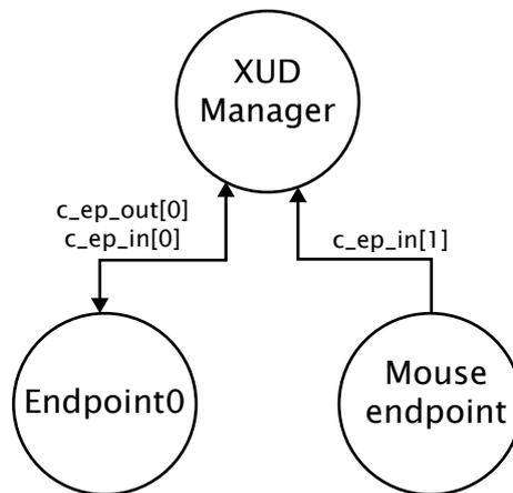
Figure 2: Task diagram of USB HID application example
