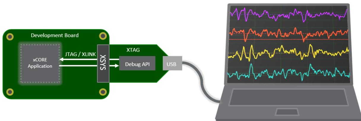
Figure 1: Block diagram of xSCOPE bi-directional endpoint example
