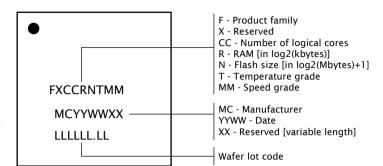
Figure 26: Part marking scheme
