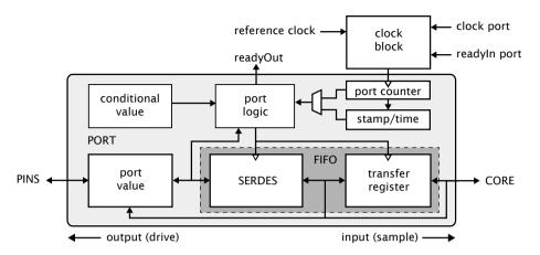
Figure 4: Port block diagram
