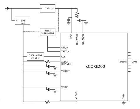
Figure 2: Simplified Reference Schematic
