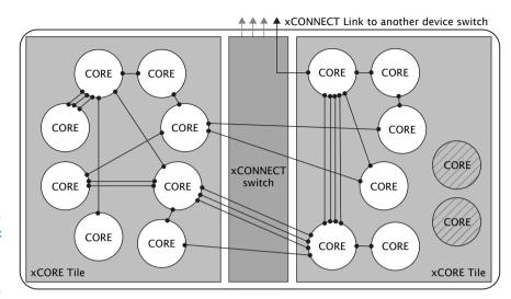
Figure 6: Switch, links and channel ends
