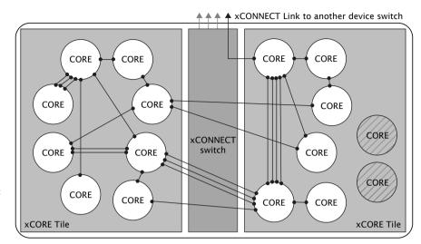
Figure 6: Switch, links and channel ends
