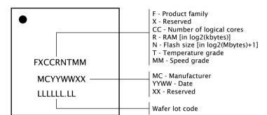
**Figure 25:** Part marking scheme
