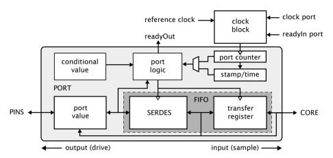
Figure 4: Port block diagram
