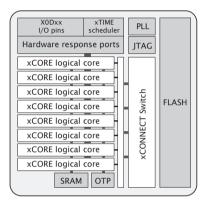
Figure 1: XLF208-128-TQ128 block diagram
