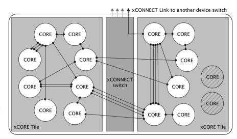
Figure 6: Switch, links and channel ends
