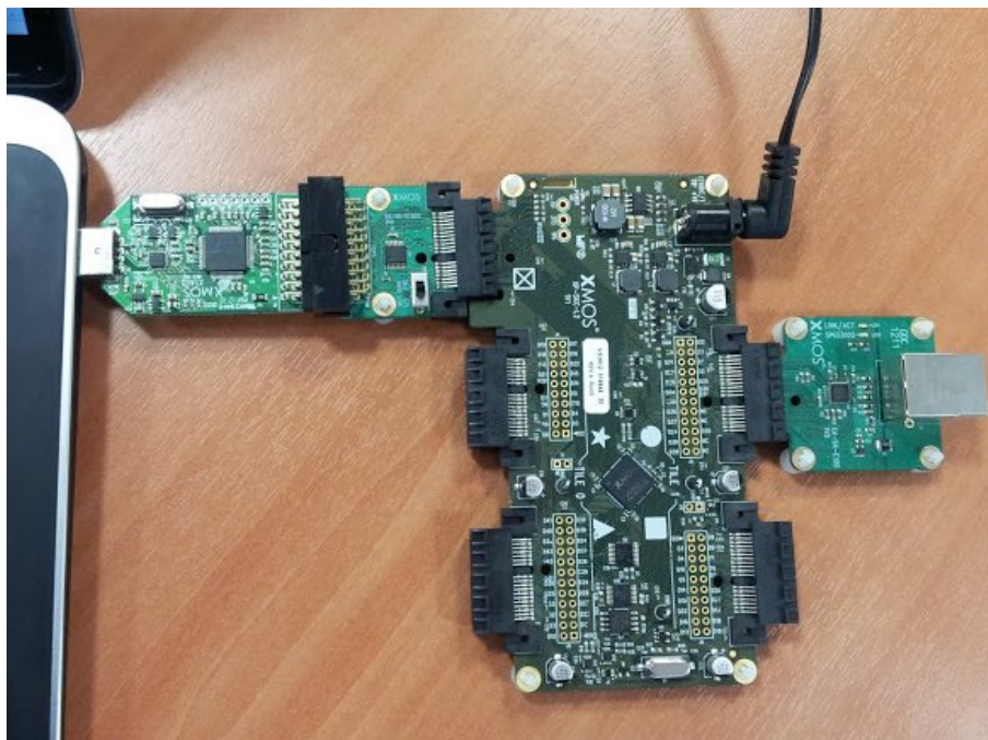
Figure 1: Hardware Setup for Simple HTTP Demo
