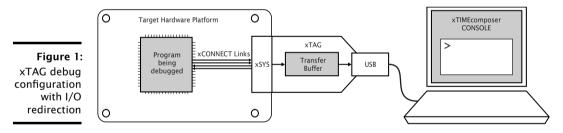
In this configuration, calls to output routines such as printf complete as soon as the data has been output on an xCONNECT Link, minimizing the effect on the program's timing characteristics. This allows debugging statements to be added to many timing-critical code sections and viewed in a console during execution. In the case of a program crash, all remaining contents in the xTAG buffer is forwarded to the PC, ensuring important information is not lost.
