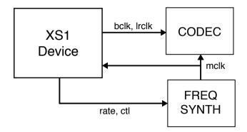
The XS1 device provides control to the frequency synthesizer and the frequency synthesizer provides the audio master clock to the CODEC and XS1 device. The sample bit and word clocks are then provided to the CODEC by the XS1 device.
