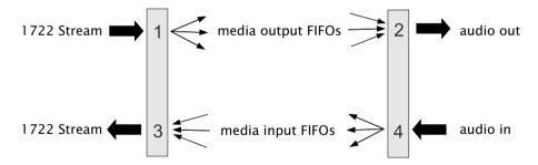
As described in the previous section, an IEEE 1722 audio stream may consist of many channels. These channels need to be routed to particular audio I/Os on the endpoint. To achieve maximum flexibility the XMOS design uses intermediate media FIFOs to route audio. Each FIFO contains a single channel of audio.
