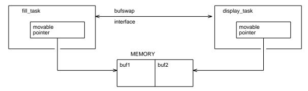
The interface between the two tasks is a single transaction that swaps the movable pointers. It has an argument that is a reference to a movable pointer. Since it is a reference the server side of the connection can update the argument.
