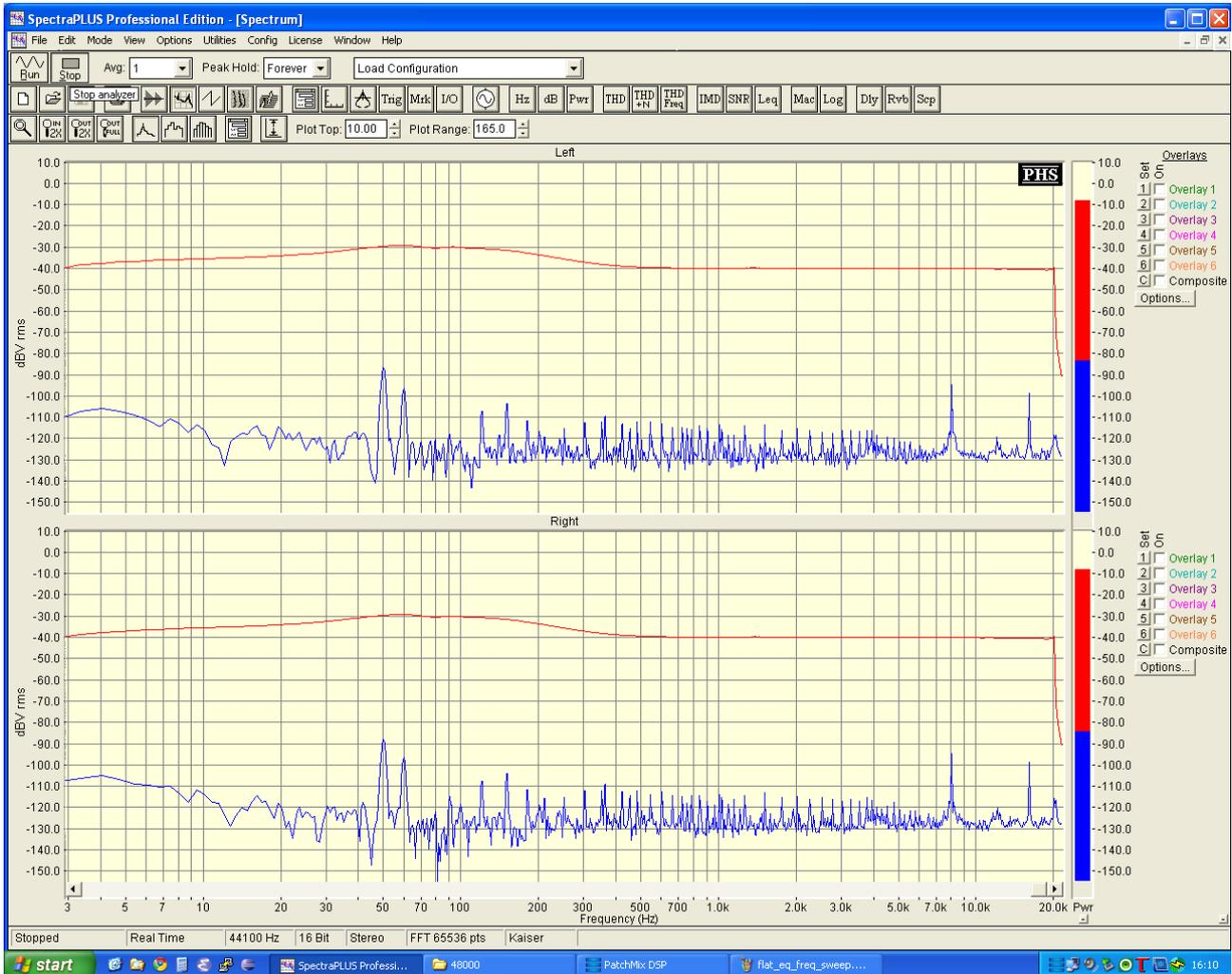
Figure 3: Frequency response for bass boost EQ setting
