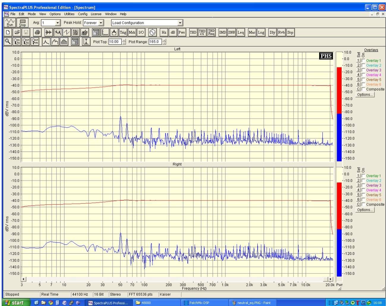
Figure 2: Frequency response for neutral EQ setting
