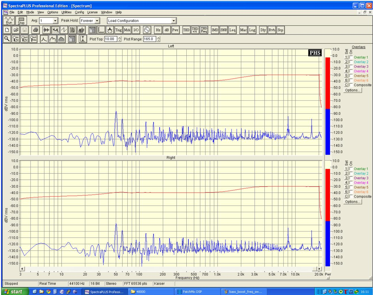
Figure 4: Frequency response for bass boost EQ setting
