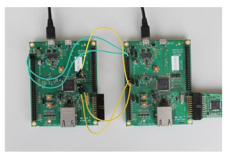
Figure 3: Connections between two eXplorerKIT boards set up as SPI slave and master
