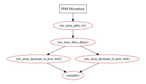
Figure 1: Application block diagram
