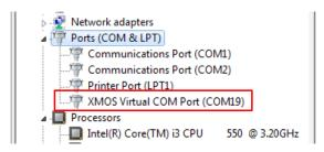
Figure 4: Enumerated Virtual COM Port Device in Windows
