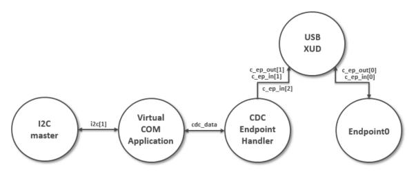
Figure 2: Task diagram of the USB CDC Virtual Serial Port example
