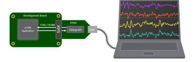
Figure 1: Block diagram of xSCOPE bi-directional endpoint example
