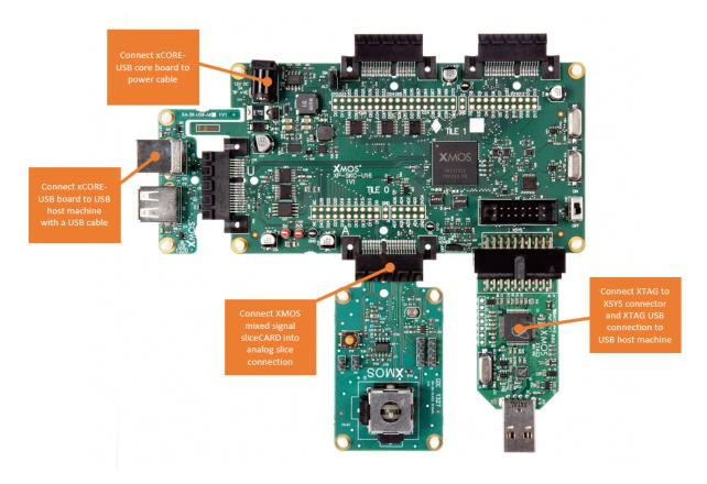
Figure 3: XMOS xCORE-USB sliceKIT
