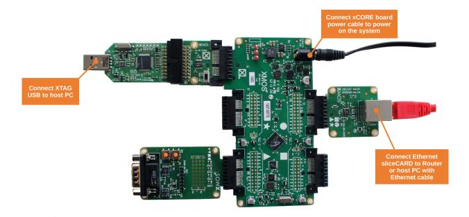
Figure 4: XMOS hardware setup for the Webserver example
