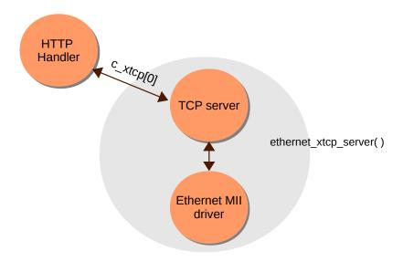
Figure 2: Task diagram of Embedded HTTP Webserver example
