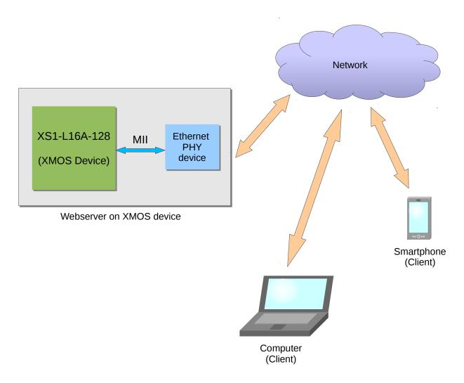
Figure 1: Block diagram of Embedded Webserver example
