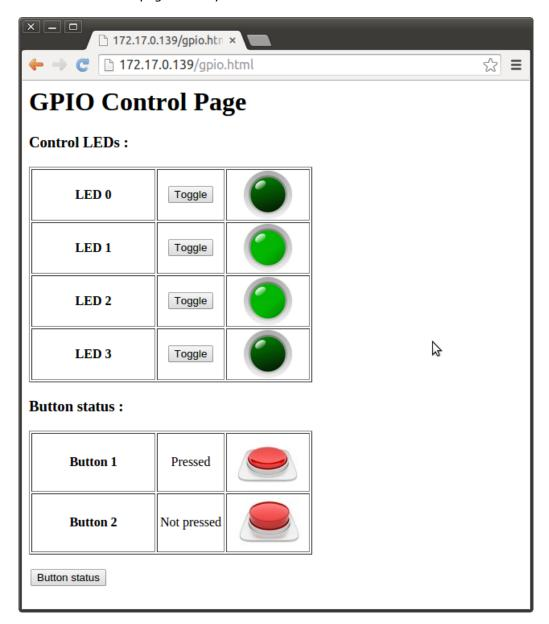
Figure 6: gpio.html page of the Embedded Webserver example
