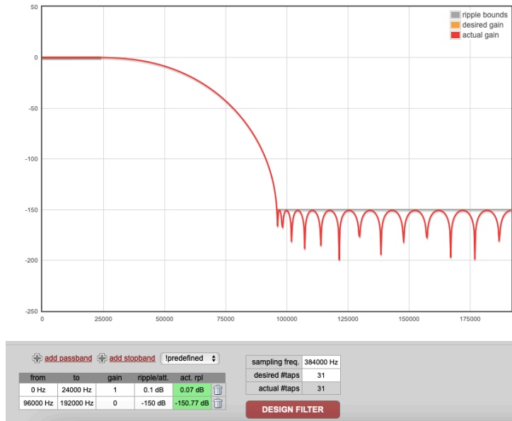
Fig. 5: Frequency response of a low-pass filter, 384 -&gt; 192 kHz.
