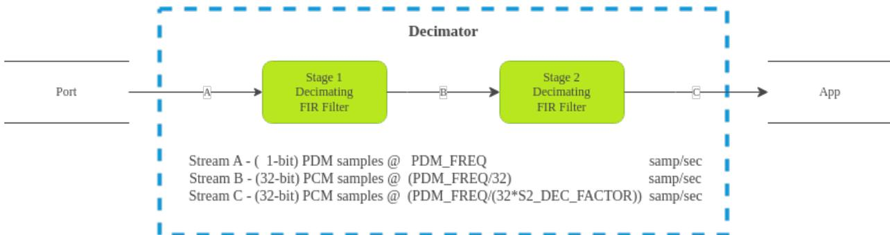
The first stage filter is a decimating FIR filter with a fixed tap count (`S1_TAP_COUNT`) of 256 and a fixed decimation factor (`S1_DEC_FACTOR`) of 32.
