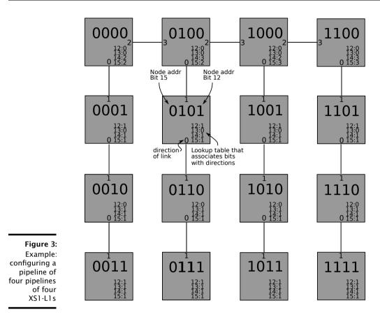
be initialised in order to use the switch. The addresses used in the configuration messages are the register numbers of the 32-bit registers in the switch.
