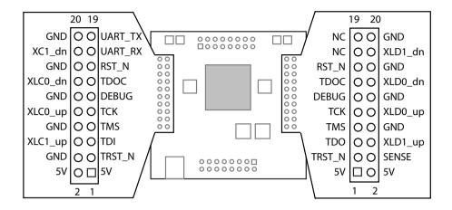
The XTAG-2 converts between XSYS and USB 2.0, allowing the XK-1A to be connected to most PCs. On power on, the XS1-L1 boots from the on-board flash memory. The XS1-L1 can then be put into JTAG mode by the PC, which then boots another program.
