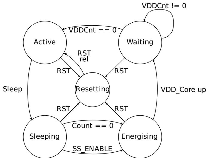
Figure 5: PCU state diagram
