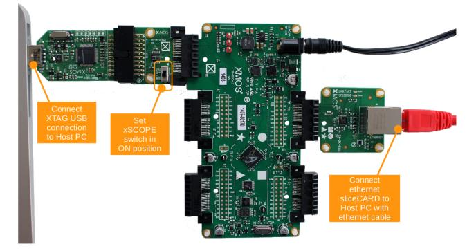
Figure 2: XMOS hardware setup for UDP demo
